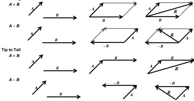
It is readily apparent that both methods arrive at the exact same solution since either method is essentially a parallelogram. It is useful to understand both systems. In some problems one method is advantageous, while in other problems the alternative method is superior.
